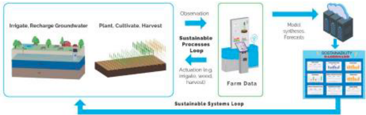
Figure 1. Illustration of monitoring, modeling, and management technology for an agricultural managed aquifer recharge (AgMAR) system, showing optimization of short-term (irrigation event) and long-term (aquifer recharge event) operations.
